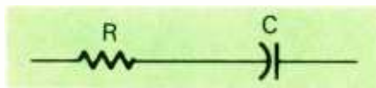
FIG. 4—FEEDBACK NETWORK used for tape playback equalization. This network is used in place of R1 , C1 , and C2 in Fig. 2.
